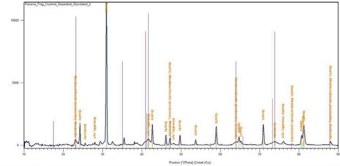
**Figure 2: XRD spectra of the ceramic body, showing peaks of montmorillonite, bentonite, hematite, and quartz**
