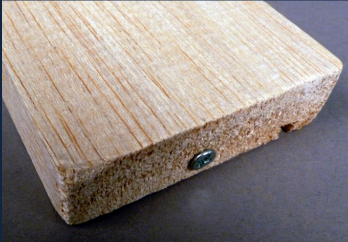
Metal screw in \frac{3}{4} " balsa wood plank
